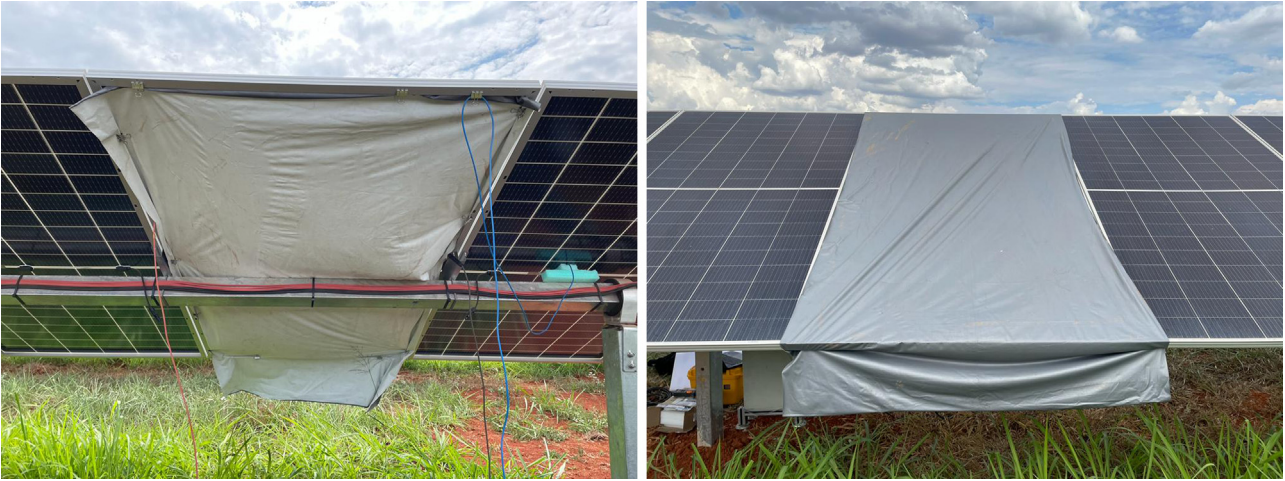
Fig. 11. Procedure for I-V characteristics of the separate front and rear sides of the bifacial module.
