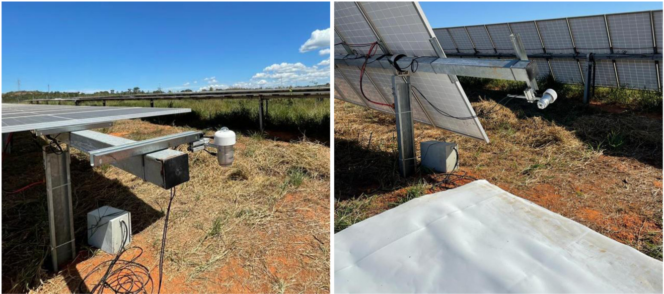
Fig. 13. Comparison measurement of albedo at Três Marias: Left – Natural ground cover; Right – Organic white sheet covering.
