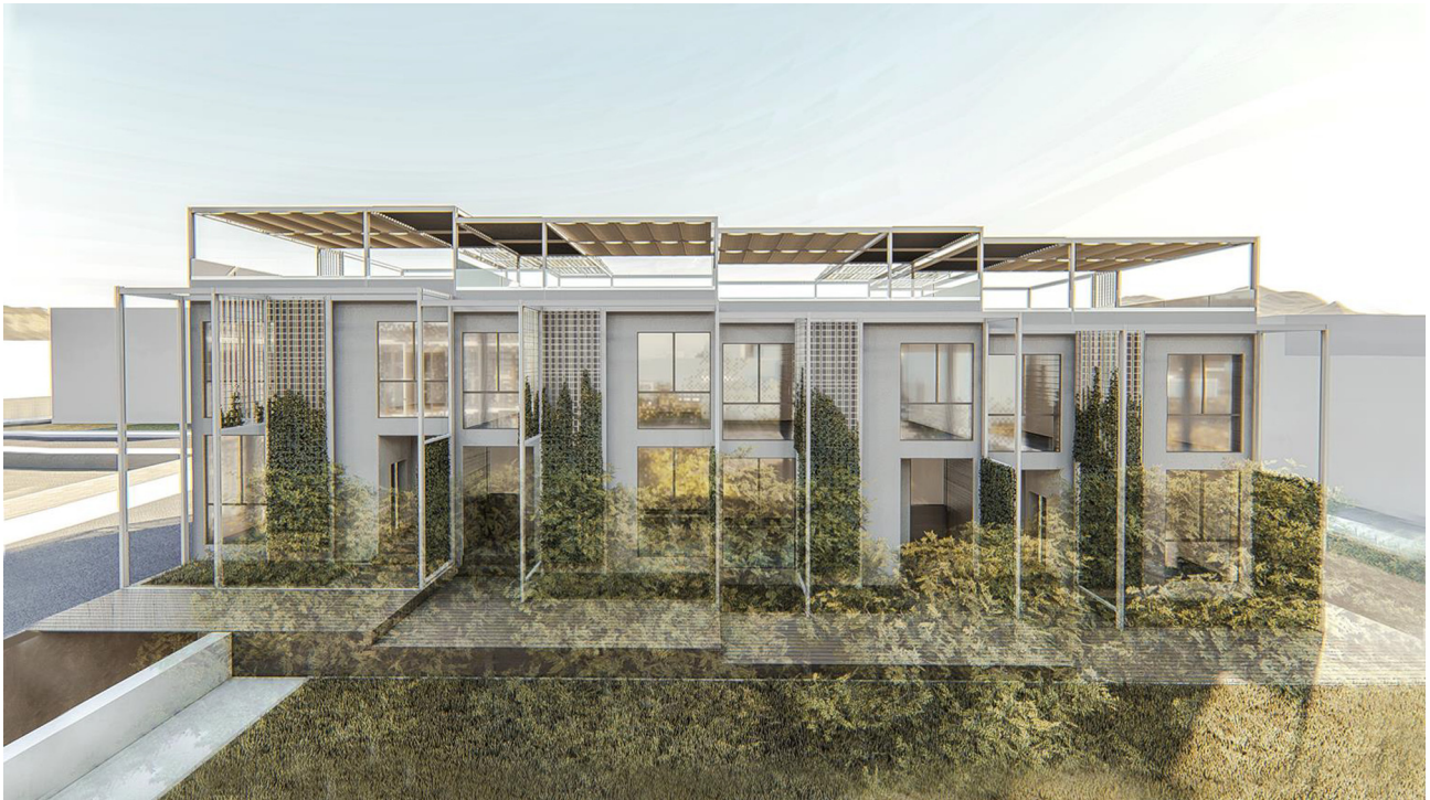
Fig. 7. Passive exoskeleton with green wind-walls made with deciduous climber plants.
