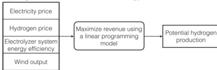
Fig. 3. Analytical workflow for estimating the potential hydrogen demand for light-duty vehicles (LDVs) and quantifying the possible production from wind energy in response to electricity market price [24].
