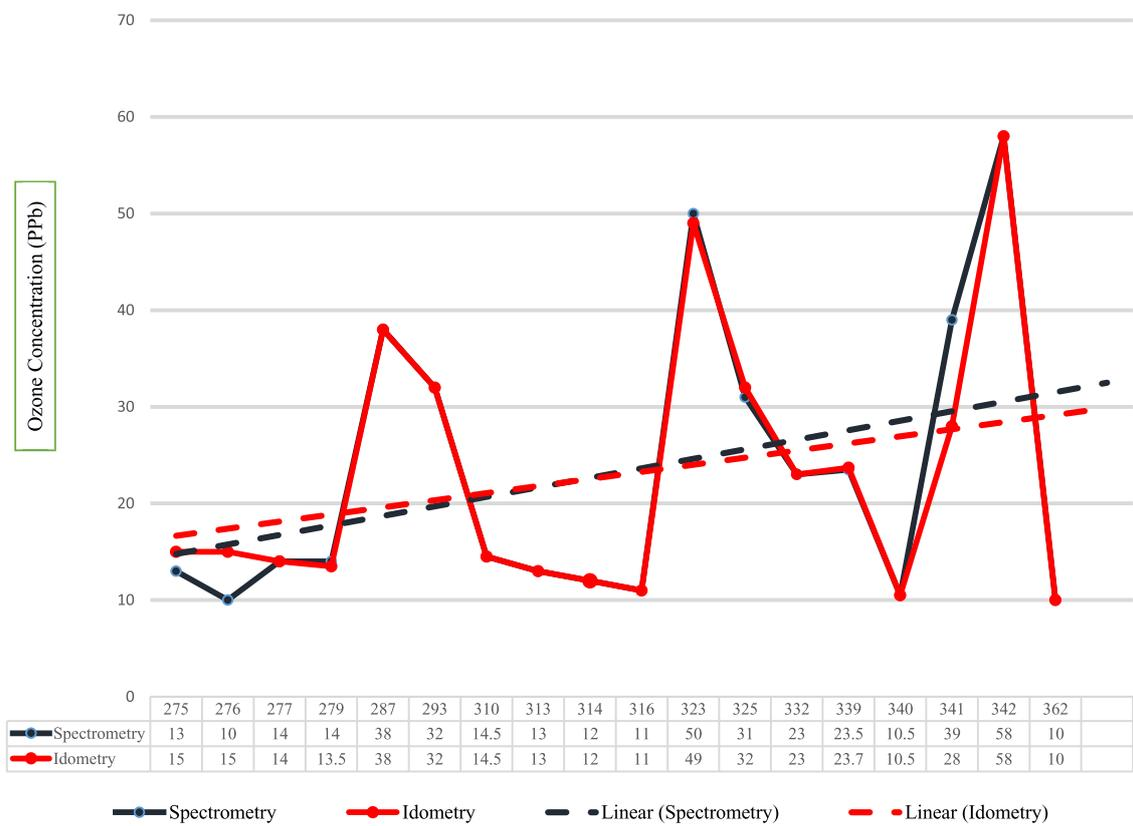
Fig. 4. Surface Ozone measurement by idometry and spectrometry method (1991–1992).
