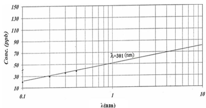
Fig. 2. Calibration via spectrophotometry method in wavelengths of 301 (nm).
