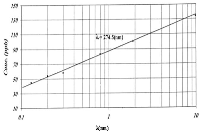
Fig. 1. Calibration for spectrophotometry method in wavelengths of 274.5 (nm).
