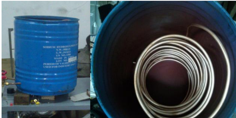
Fig. 2. Copper coil of new condenser.
