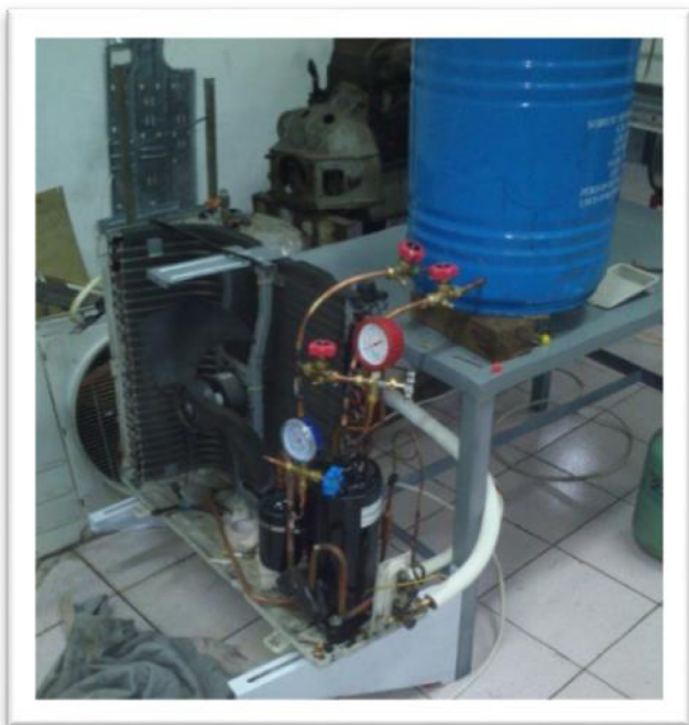
Fig. 3. Modified AC system with a new condenser.
